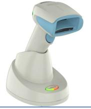
**Cordless Barcode Scanner Set-up**: With the first use, the scanner <u>must</u> be linked to the base. Scan the pairing bar code that is located on the back of the scanner base. The scanner will automatically initiate the linking process without placing the scanner into the base. Once finished, the scanner will emit a single beep. This is a one-time set-up only.
